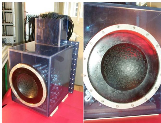
Figure 6. The 200-element sparse array prototype and the electronic system. The waterproof PVC cube contains the 200 electrical matching boxes. On the right: the quasi-random distribution of transducers embedded in spherical shaped Ureol.
