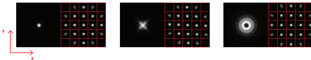
Figure 3.3 – Illustration of parsing into 5 \times 5 sub-apertures for a point source without any aberration, with astigmatism and with defocus (from left to right). For each part of the illustration, the first image represents the point source in the image plane. The second image represents the sub-images in the image plane. Every focal spot is in the center of each sub-image when there is no aberration. Each aberration is associated to a set of sub-image shifts.
