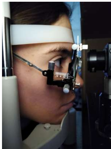
Figure 3.13 – Photo of the verification experiment. Astigmatic glasses are placed and adjusted in front of the emmetropic eyes using holders.
