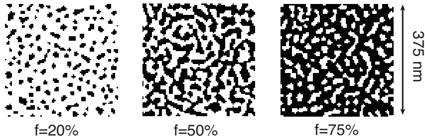
Figure 3.2: Numerically generated gold films for three different filling fractions f (gold is represented in dark). The parameters for the computation are: T = 300 K, \alpha = 2 \times 58.10^2 , F = 1014 \text{ s}^{-1} , A = 0.2061 eV, B = 1.79 eV, p = 10.229 , q = 4.036 .
